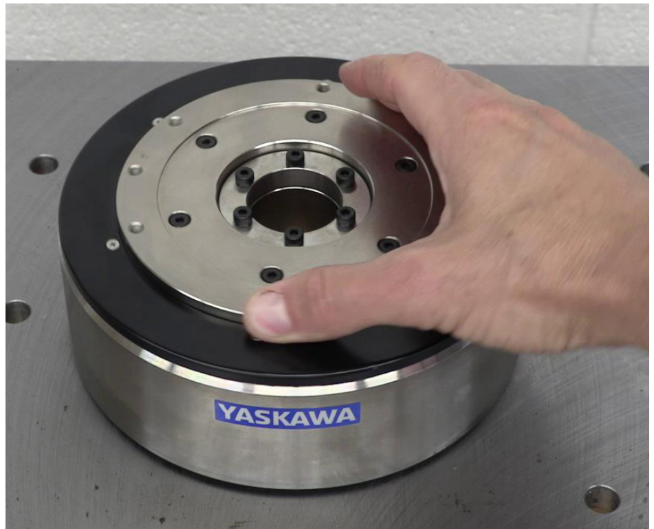
Figure 1: A typical direct drive motor mounted on a steel plate
