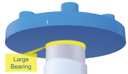
Figure 13: The large bearings of direct drive motors increase load capacity.
